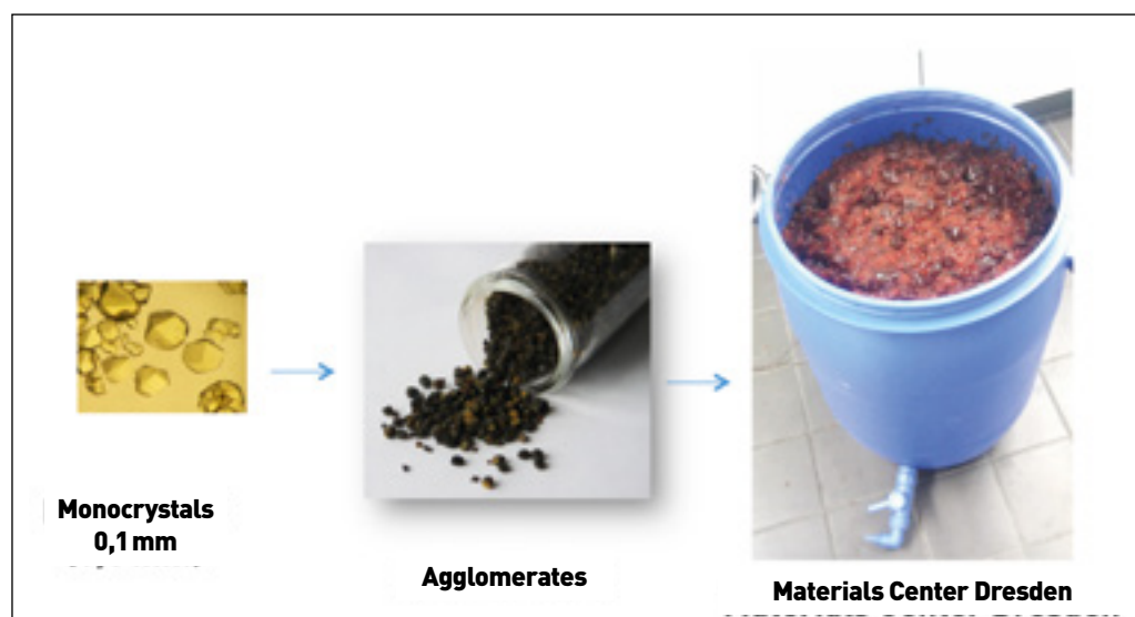
Fig. 6 Scaling-up of MOF production in Dresden up to the 10 kg scale
