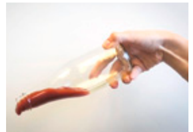
Ketchup slides out of a bottle that has been coated with LiquiGlide.
